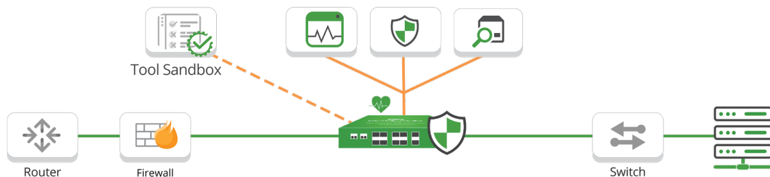
Diagram 2. Managing multiple inline devices, while sandboxing a new tool
