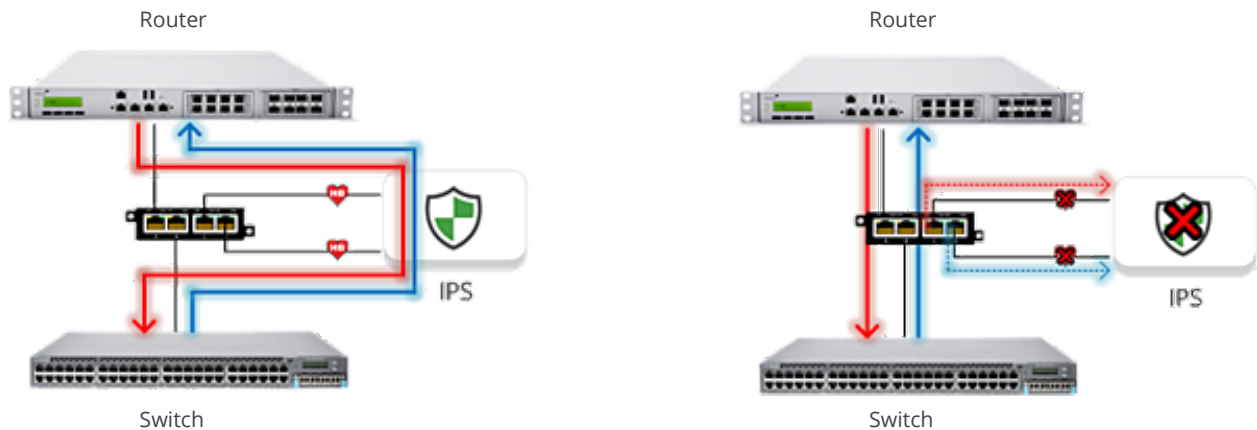
Diagram 3. Taking an IPS inline and out-of-band using a bypass TAP
